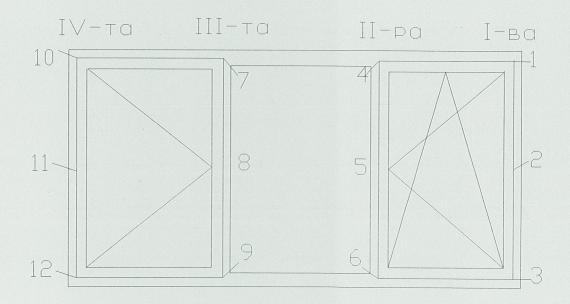
Disposition scheme of measuring points on the window
